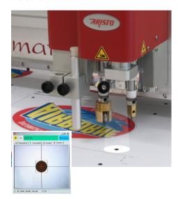
Live image on the PC monitors shows placing and adjustment of the fiducials and/or in the simulation mode the cutting outlines.
