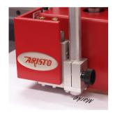
Installed at the tool head the pneumatic marking module works as an additional tool. It is possible to mark or label the production pieces without tool change.
