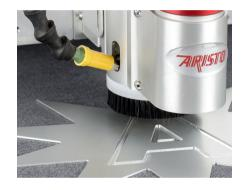
Materials that are not easily machinable without a cooling lubricant, or where there is an increased tool wear, can be milled with a minimum quantity of cooling lubricant.
